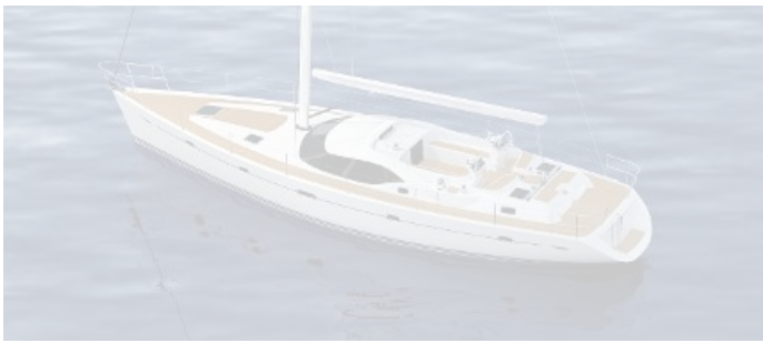
Oyster 575 (16 C 58): 19-metre sloop with an optional lifting keel.
